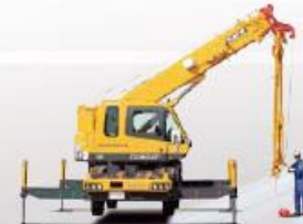
Drop auxiliary hook, boom down, secure auxiliary rope to Fly Jib
