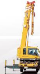
Telescopic boom extended to release Fly Jib
